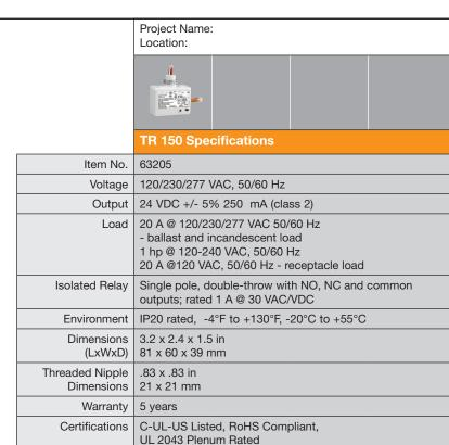
The TR 150 is a full featured power pack with an isolated relay that provides power to STEINEL low voltage occupancy sensors and other control devices. They are Class 2 output power supplies, suitable for parallel interconnection.
