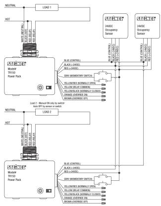
Upon occupancy, lights (Load 1) attached to Power Pack (set to Auto ON) will illuminate automatically while lights (Load 2) attached to Power Pack (set to Manual ON) require the occupant to turn the lights on manually by means of a low voltage switch. All lights can be turned off manually by a low voltage switch or automatically by an occupancy sensor(s).
